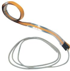
The tape sensor is 2 meters long and is attached to a 1 meter cable. The tape sensor can be glued to a smooth, clean floor surface such as a painted, lacquered or plastic-coated floor.
