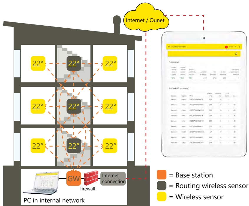
FIGURE 1 structure of wireless sensor network
