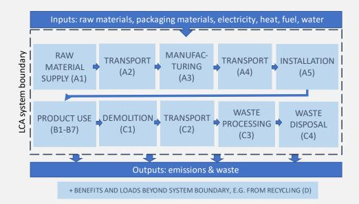
**Manufacturing (A3):** Manufacturing and packaging of the products. The assessment covers the electricity and heat consumption needed in the production process and the transport and management of production waste. The electricity is modelled with national residual mixes in the absence of the guarantees of origin. The district heating (production mix) is modelled site-specifically with the information provided by energy companies.
